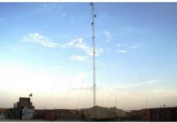
The Mobile Communication Unit consists of a 30-meter transmission mast constructed on a trailer. This makes it a multipurpose system that can be deployed wherever necessary.
