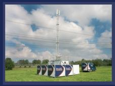
COW – Cell on Wheels A ready to deploy, mobile and multi-purpose total solution with a 25 meter high mast
